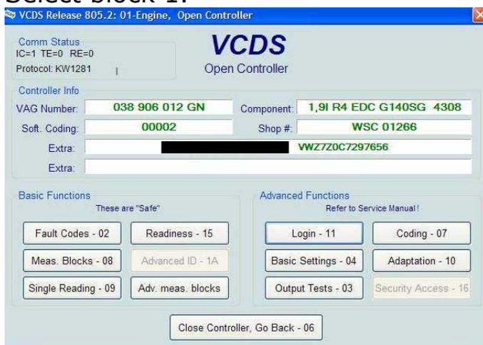
Block 1 should show the IQ. The IQ value is normally about "3.0-5.0 mg/str". If the IQ is bouncing around as much as 1 to 6 then the engine isn't warmed up or there's either an injection pump internal fault or ECU fault. The default adaptation number, whether you have a chip or not, is 32768. A lower adaptation number entered in the blank will reduce fueling and increase the "x.x" m/R value. A higher adaptation number entered will increase fueling and lower the "x.x" mg/R value.
